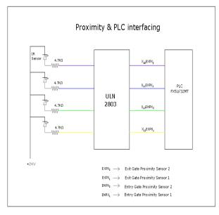
Fig. 2: Wiring diagram for PLC and Sensor interface
