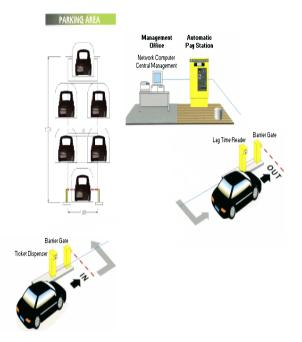
Fig. 4: Schematic view of overall parking system
